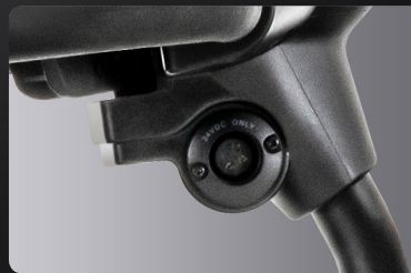
Charger port located conveniently on the tiller.
