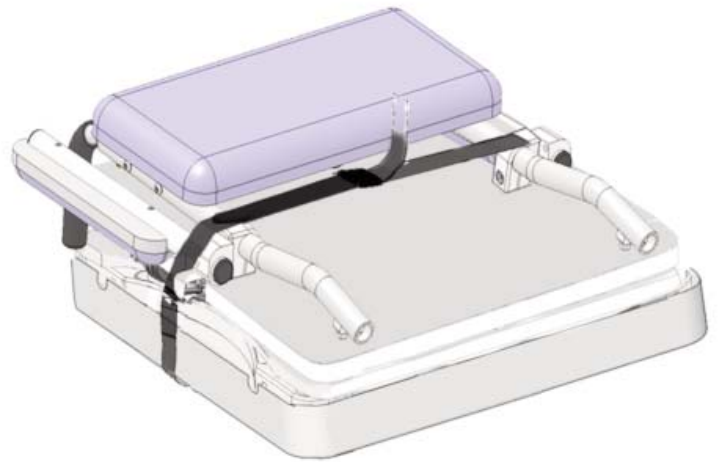
Figure F - Tighten & buckle the black strap around the inverted frame & backrest assembly.
