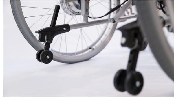
Anti tippers on the Model X fit into the tube behind the rear wheels
