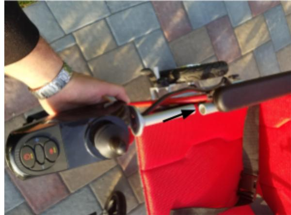
Attach the Cord into the Clips running to the back of the chair
