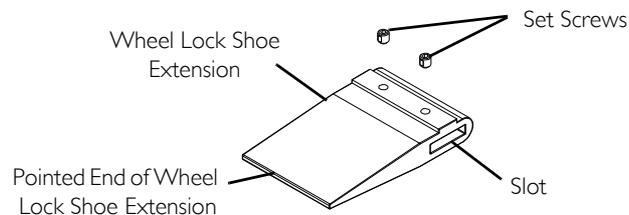
**FIGURE 9** Installing Wheel Lock Shoe Extensions
