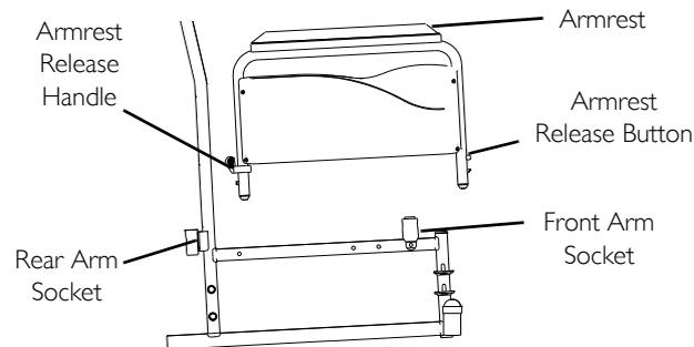
**FIGURE 6** Removing/Installing Armrests
