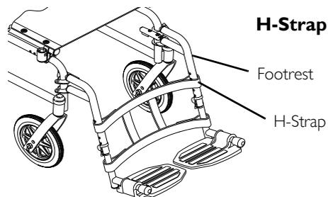
**FIGURE 8** Installing H-Strap/Calf Strap
