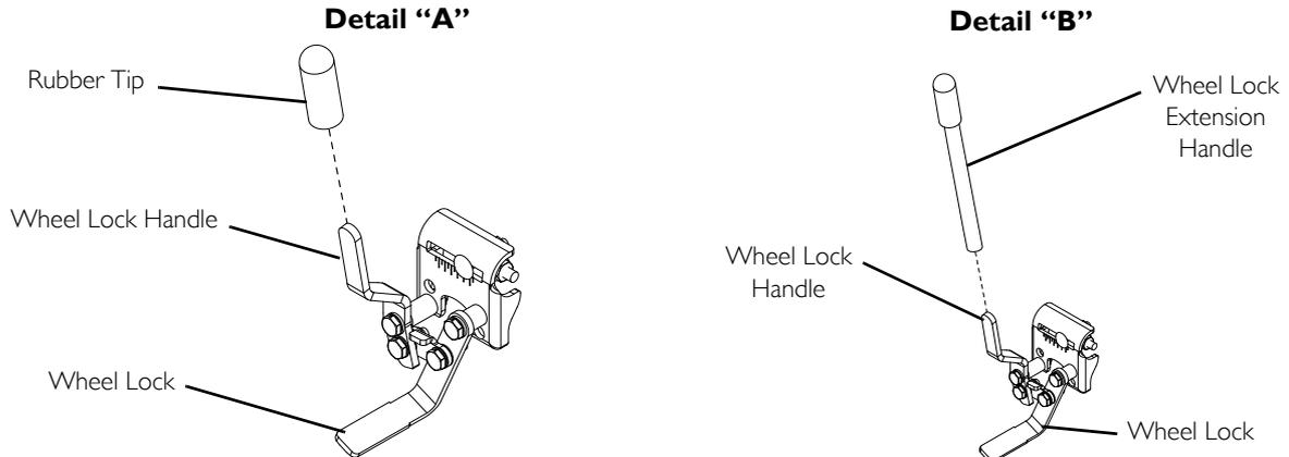
**FIGURE 9** Installing the Optional Wheel Lock Extension Handle
