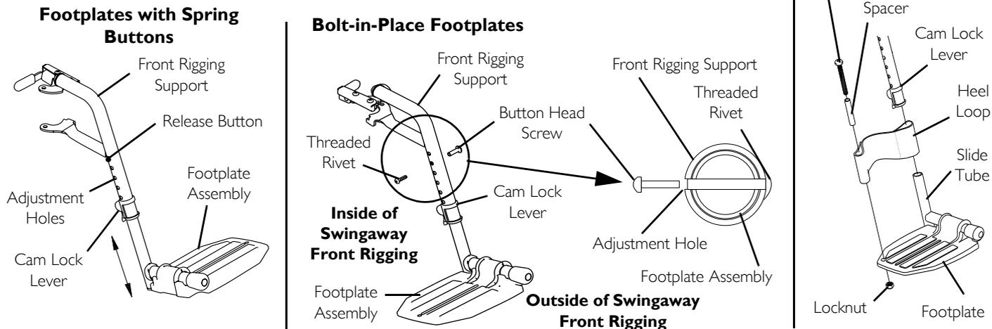
**FIGURE 1** Replacing Heel Loop
