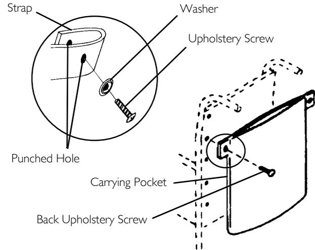
**FIGURE I** Installing Carrying Pocket
