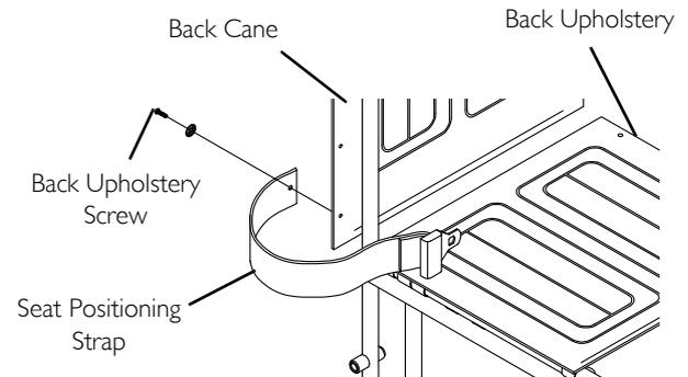
**FIGURE 3** Installing the Seat Positioning Strap
