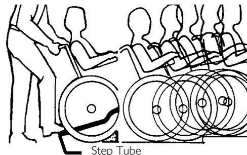
**FIGURE 2** Method 1 - Wheelchair With Step Tubes
