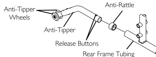
**FIGURE 7** Installing the Anti-tippers
