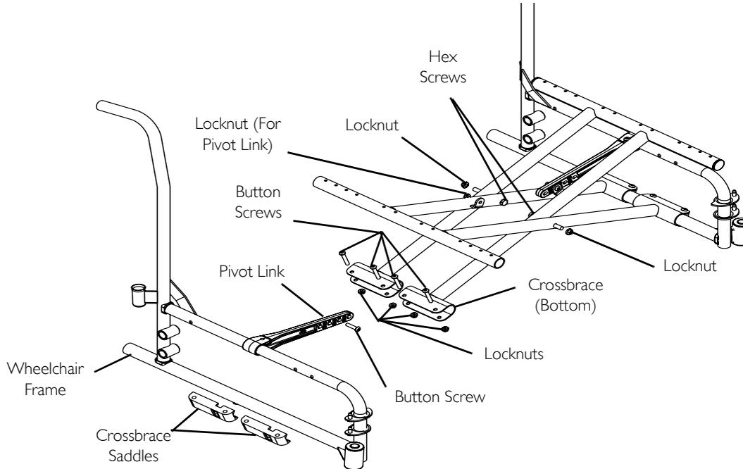
**FIGURE 3** Adjusting the Seat Width
