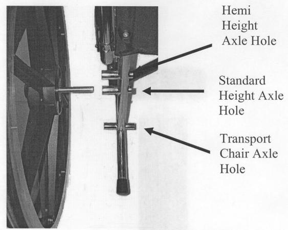
**Step 1:** Depress the quick release button on the wheel hub and pull off the wheel and quick release the axle from the standard height axle hole.
