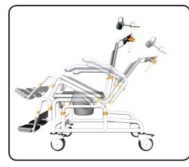
While squeezing the brake handle the chair can be reclined 30° from upright.
