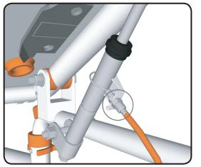
Check to ensure that the cable adjustor is screwed all the way in as shown.
