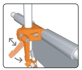
After adjusting the neck rest you can adjust the position of the neck rest handle to prevent it sticking out.
