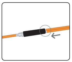
Check to ensure that the stainless steel caps on the ends of both of the orange cables are inserted all the way into the cable adjustor as shown. During packaging/shipping and owner setup these parts can sometimes come out.
