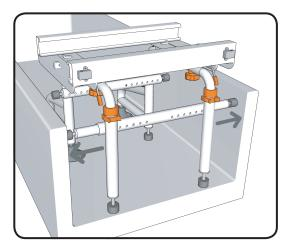
With the bath base in the bath and correctly adjusted, secure it in position by adjusting the stabilising tubes.
