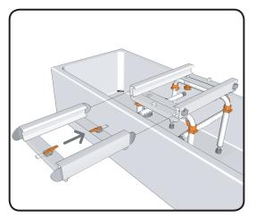
Align the bridge with the bath base and insert the tongues into the bath base.
