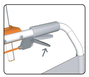
To return the chair to an upright position squeeze the tilt handle on the left hand side of the back rest.
