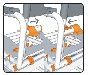
By sliding the armrest lock you can easily swing the armrest out of the way or secure the armrest in position.
