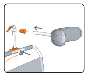
To attach the neck rest, insert the plastic sleeve into the neck rest height adjustment tube.
