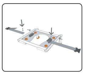
Insert both height adjustment tubes into the bath base legs. Ensure the holes on the height adjustment tubes align with the holes on the bath base legs.
