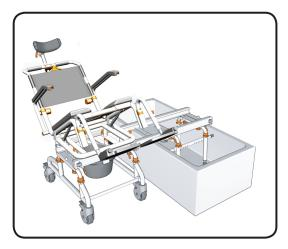
Securely attach the bridge to the bath base using the latches. Next securely attach the bridge to the wheeled base using the latches.
