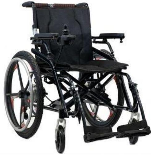
Slip in the battery underneath the seat
