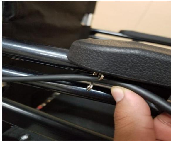
Before folding the chair make sure to release the back handleBar
