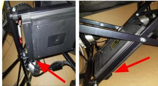
Make Sure The wires under the seat are connected properly.
