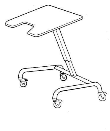
The Tristander Tray 45 is height adjustable from 24 - 36 inches. The Tristander Tray 58 is height adjustable from 34 - 49 inches. To adjust the height pull the plunger pin and slide the tray top up or down
