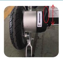
Pull down to change to manual mode; pull up to change to electric mode
