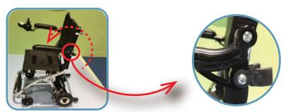
Grasp arms at their ends and rotate up and forward until they contact the stopper on the back post
