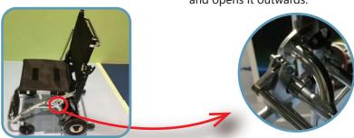
Make sure the frame is open and in place, and try to push the wheelchair and check it shake or fall off.
