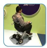
By pushing the joystick, the user operate the wheelchair and arbitrarily in any direction
