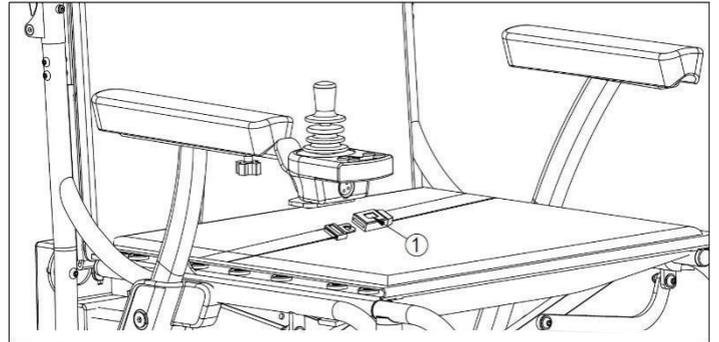
Figure 11. Positioning Belt Adjustment
