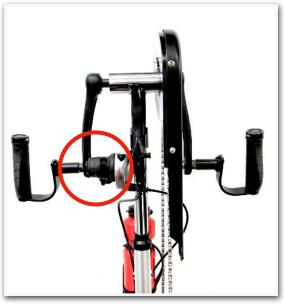
The shifter should not be level w/ the pedal QR pin.
