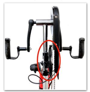
The location is good but the brake lever is too close to the chain. There should be at least 1/2" / 12mm minimum between the brake lever and the chain.
