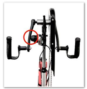
The shifter should not touch the inside of the left crank arm.
