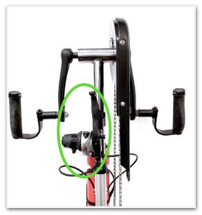
The bracket should be low and near the fork clamp. This gives 1" / 25mm clearance between the shifter and left crank arm. There is clearance to access the parking brake.
