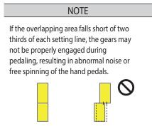
3) Adjust the shifter barrel adjuster if necessary to realign the 2 yellow lines.
