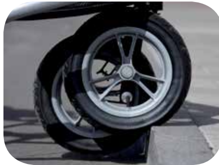
The Trionic Climbing Wheel in action climbing a 5 inch high curb
