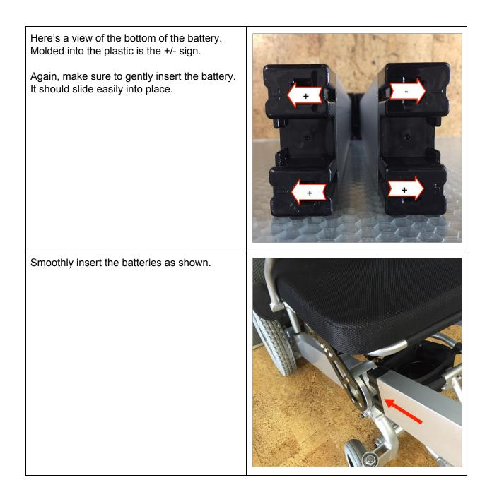
To remove the batteries, pull out evenly while depressing the plastic clasp on each side.
