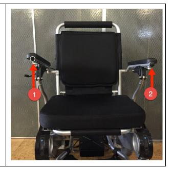
Slide the controller into the open slot as shown.
